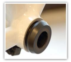
Confirm that all clips and bearings are installed into BB30 bottom bracket shell. Identify left and right side adapters and start inserting the adapters into the bottom bracket by hand.
