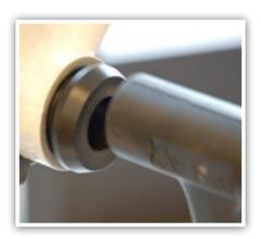
2. Seat adapters using a rubber mallet.
