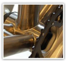
3. Install crank spindle through adapters and tighten per manufacturer's instructions. Take up any play in your cranks with our Crank Spindle Spacers and place as shown above.
