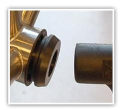
2. Seat adapters using a rubber mallet.
