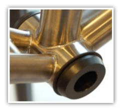
If not already installed, press the PF30 bottom bracket cups into frame. Identify left and right side adapters. Remove outer dust covers, if present. (Do not remove the bearing seals). Start inserting adapters into bottom bracket bearings by hand.
