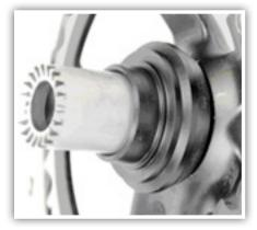
Confirm that all clips and bearings are installed into BB30 bottom bracket shell. Identify left and right side adapters.
