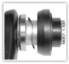
Install right adapter into the 6806 bearing on the right side of the bottom bracket. Tap into place with a soft-faced mallet. Push right crank with its factory-installed bearing in to the right adapters. Tap into place.
